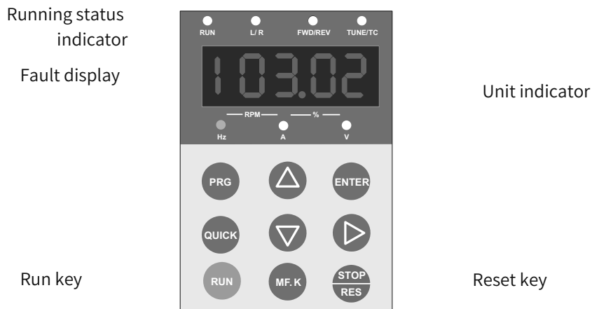
Figure 7-2 LED display of a fault
